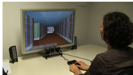
Figure 5: A faceLAB eyetracking system monitored participants’ eye movements during the interactions.
