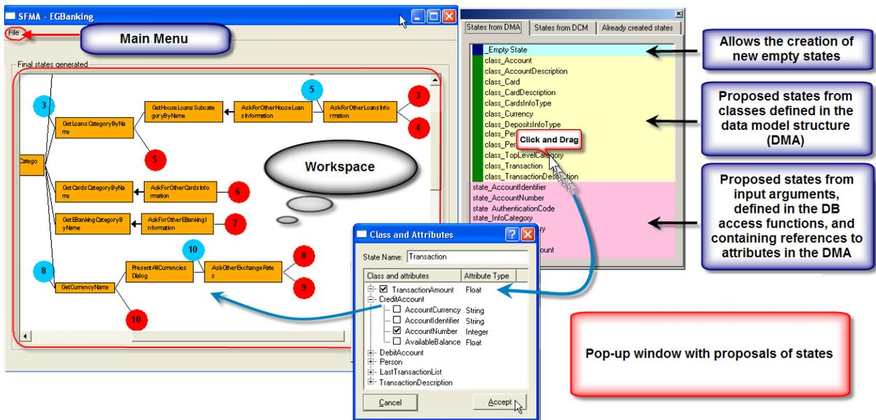
Figure 6. Workspace for creating the state transition network and pop up window with state proposals. In the example, the designer creates the state *Transaction* from the *Class\_Transaction* template (created in the DMA, see Figure 2) and selects as slots the *TransactionAmount*, *CreditAccountNumber* and *DebitAccountNumber* (not shown)
