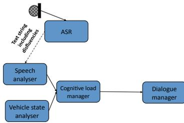
Figure 2: Architecture of the cognitive load manager.
