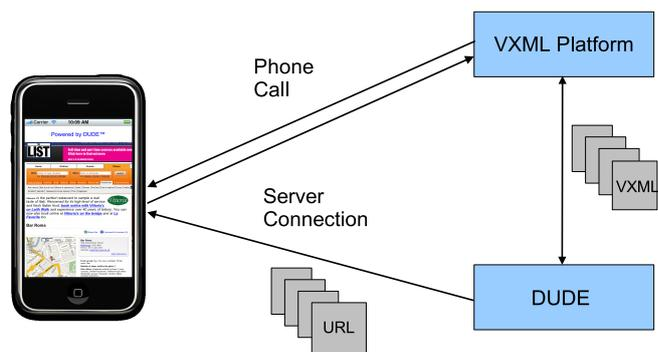
Figure 5: Architecture of deployed DUDE Application on a mobile phone (e.g. the iPhone)
