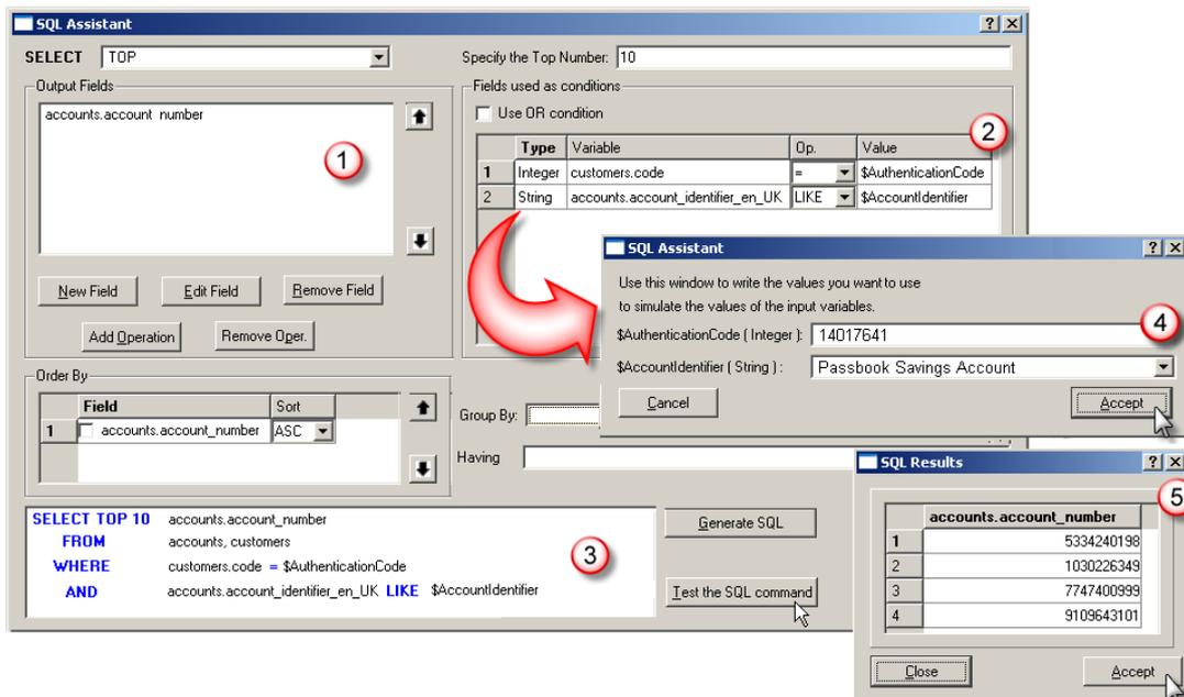
Figure 5. Wizard for creating and debugging the SQL statements for accessing the backend database. In the example, the proposed query allows the selection of all account numbers for a given customer (using his/her authentication code) and type of account (i.e. passbook saving accounts)
